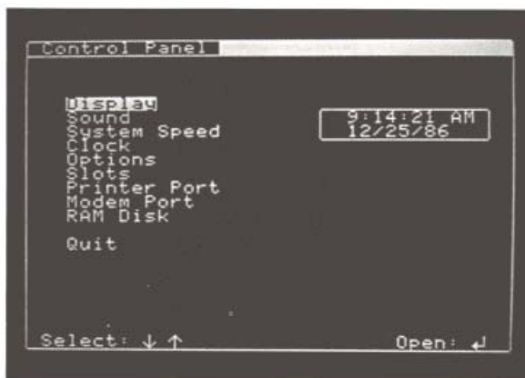
Figure 3-3 Control Panel Program Main Menu
