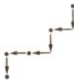
Figure 4. Vectors for a diagonal line
