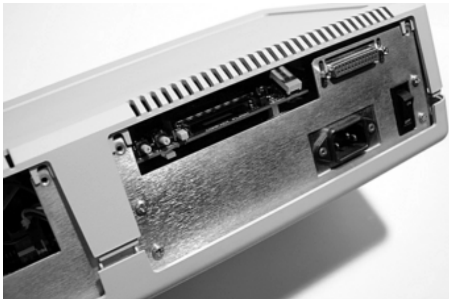
Figure 53. Initial location for replacing the top cover
