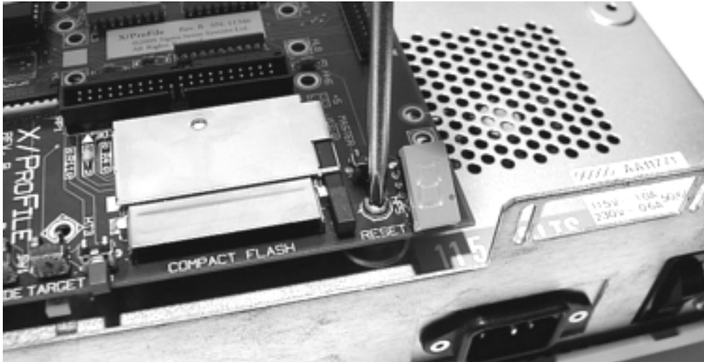
Figure 43. Inserting the grounding screw
