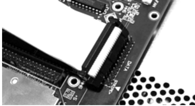
Figure 45. Connect the data cable to the X/ProFile with the stripe near the triangle
