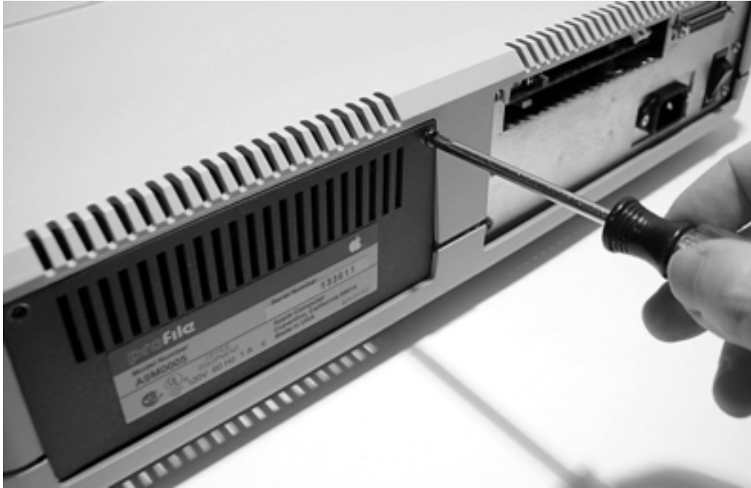
Figure 55. Replacing an escutcheon plate
