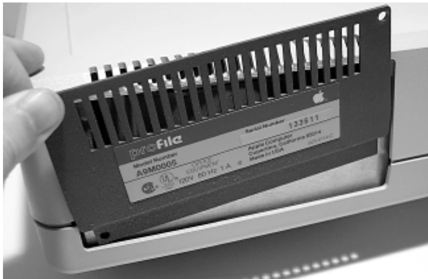
Figure 6. After removing the screws, the escutcheon plate is lifted out
