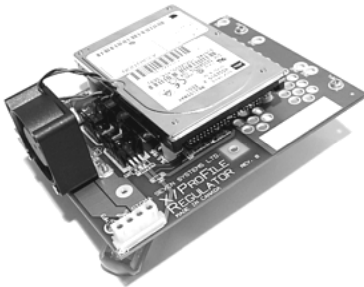
Figure 32. A 2.5" drive mounted to the X/ProFile Regulator
