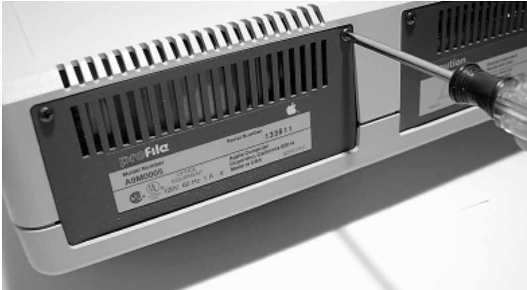
Figure 5. Removing the escutcheon plate screws
