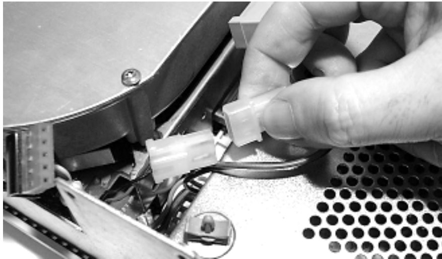
Figure 21. Disconnecting the two-wire hard disk power connector
