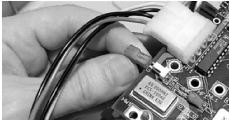
Figure 52. Re-connecting the READY LED cable
