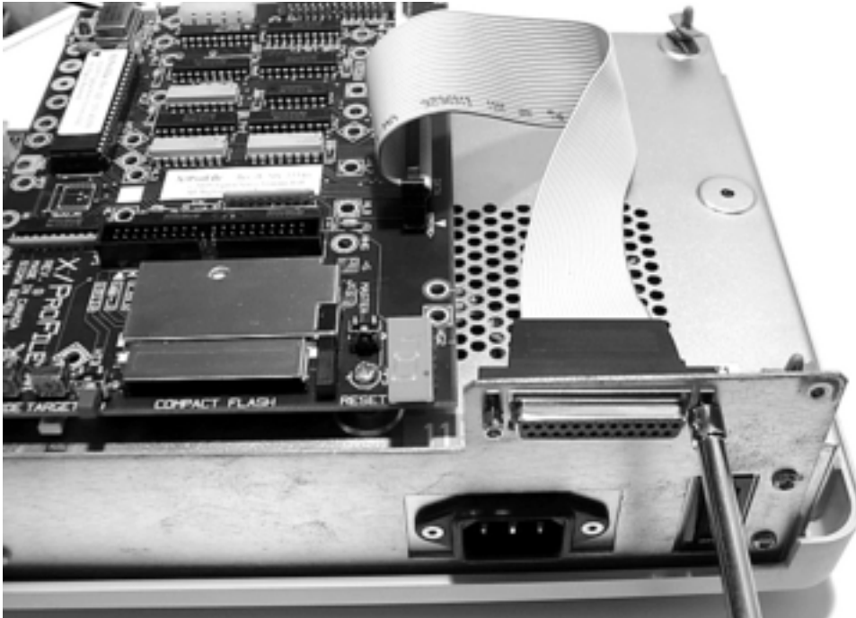
Figure 47. Attaching the DB-25 connector to the chassis back panel
