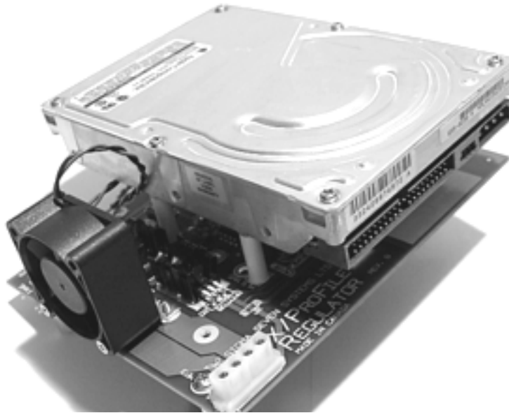
Figure 30. A 3.5" drive mounted to the X/ProFile Regulator
