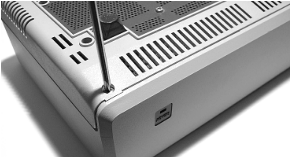
Figure 4. Removing the top cover screws
