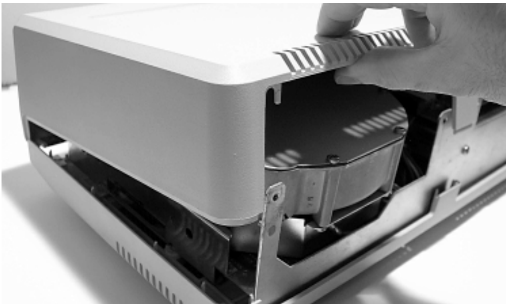
Figure 8. The top cover comes free after the latches at the front disengage
