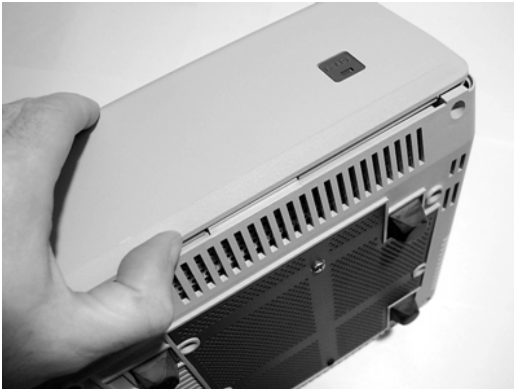
Figure 54. Engaging the latches along the front edge
